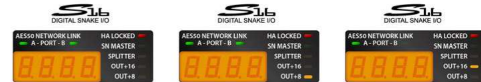
FOH console supplies clock synchronization and controls the S16 preamps exclusively (local HA control is blocked by console)
